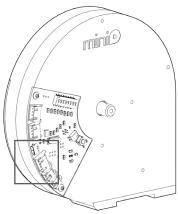
Use provided wire to connect sensor into the electronic board.
