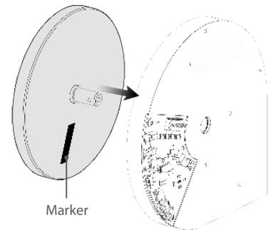
**Note:** Make sure the marker (black tape) is facing the electronic board.
