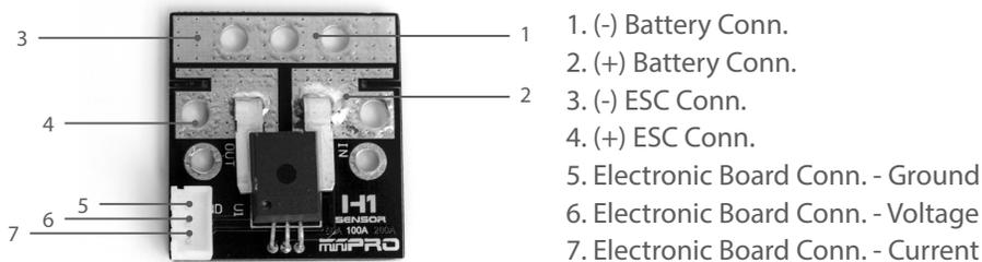
NOTE: This diagram applies to the 50A, 100A, 150A and 200A sensor.
