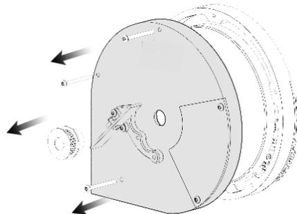
**Note:** Need to remove the pulley first before removing the front cover.
