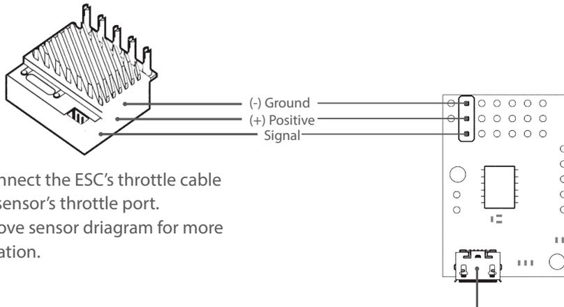
2.1. Connect the ESC's throttle cable to the sensor's throttle port. See above sensor driagram for more information.
