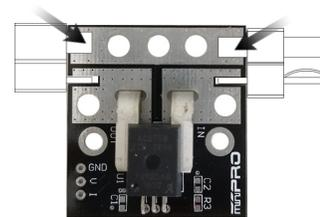
Solder the connectors of your preference OR 14 gauge wires. Try to keep the wires as short as possible to reduce the electrical losses
